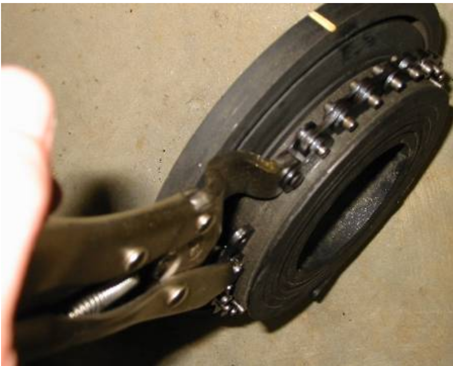
11.) Use Chain Wrench to hold crank pulley while using 6 foot breaker bar to remove Main Crank Pulley.
