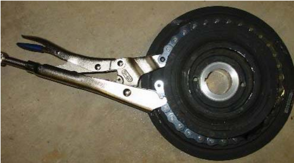
11.) Use Chain Wrench to hold crank pulley while using 6 foot breaker bar to remove Main Crank Pulley.
