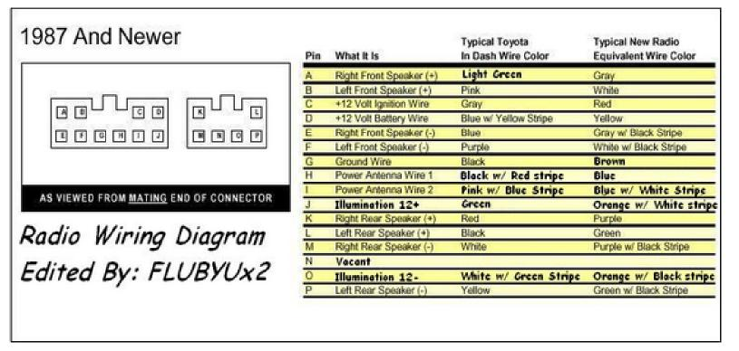
The black on the toyota in-dash wiring is NOT chassis ground. it is one of the terminals for the rear speaker, the other terminal being YELLOW.
